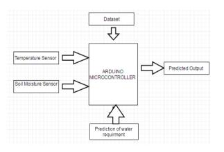
In this System We have used Dataset to calculate the Prediction of Crop Planning using the hardware sensor like Temperature Sensor and Soil moisture Sensor .Senses data is further send over Arduino to Computer /Machine .We will apply the Dataset and can predict the planning of crops will planted in the farm or land.
